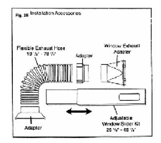
Customer could select and assemble the *Exterior Wind Suction Adapter* - a tube that draws in fresh air from outdoors, which cools down the condenser. The installation is as following figure.
